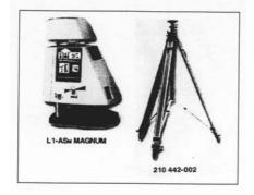
TECHNICAL CHARACTERISTICS Minimum height of operation...±1, 57 (m) Maximum height of operation .±3,98 (m) Height of folded tripod......1,83 (m) Weight.....±13 (Kg) Tripod head.....level ø 110 (mm) Telescopic part.....2-part Distance of telescopic part....595/600 (mm)
