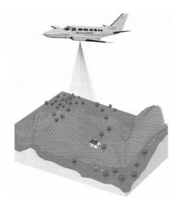
Figure 1.The principle of the airborne laser scanning.
